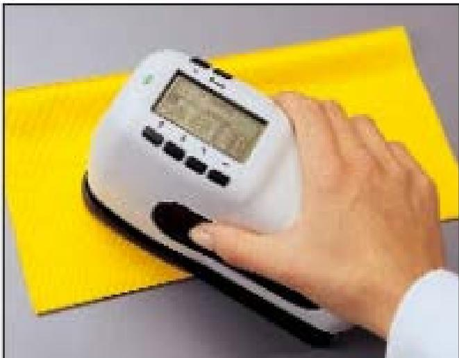
*A portable sphere spectrophotometer measures the color of textile samples and other materials where the product's appearance is critical for buyer acceptability.*
