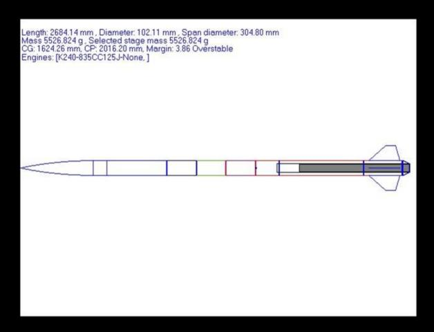
Fig. 3. Simplified Rocksim schematic of the Flying Bison. Left to Right: Nose cone, main parachute bay, forward electronics bay, drogue parachute, aft electronics bay, motor mount & fin can
