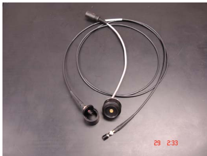
Fig. 7. Plume emission monitor with Silicon Photodiode and Amplifier and fiber optic cable terminated in with lens on each end.
