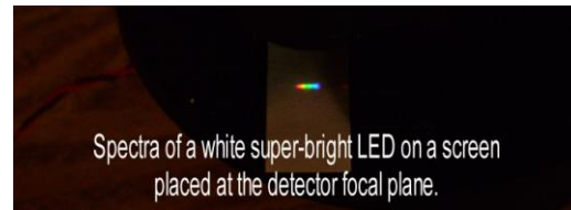
Figure 4.6 Spectrum of Super-Bright LED at the focal plane. The spectrum is clearly visible with red on the left and blue on the right.
