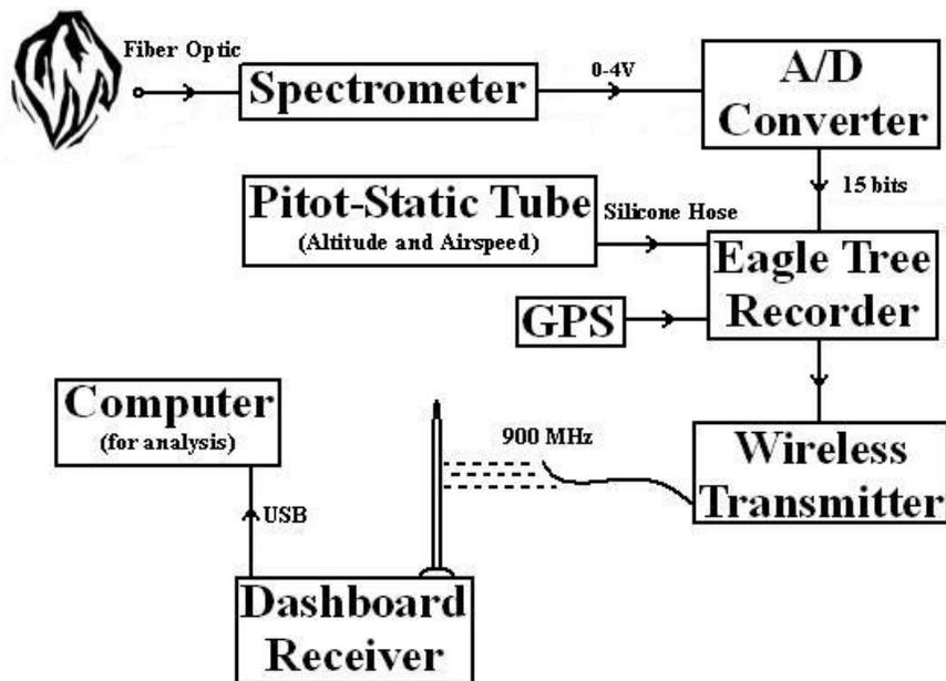
Figure 4.7 Schematic of microcontroller subsystem.
