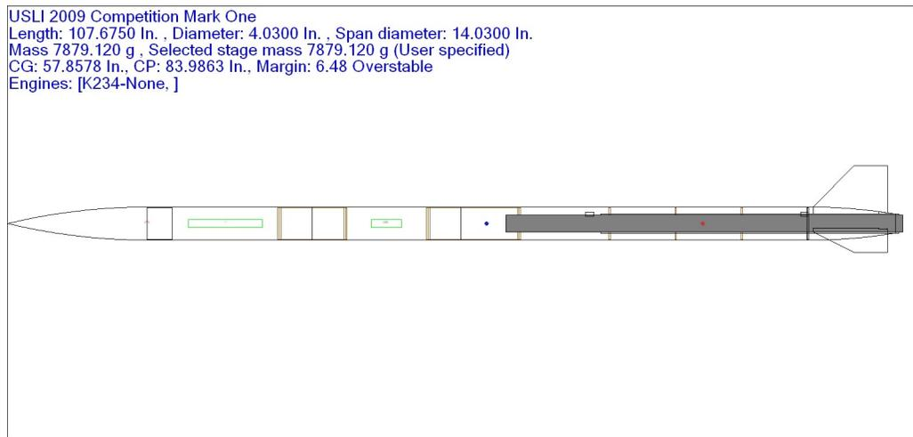
**Figure 3.6: Competition Rocket Stability Diagram.**
