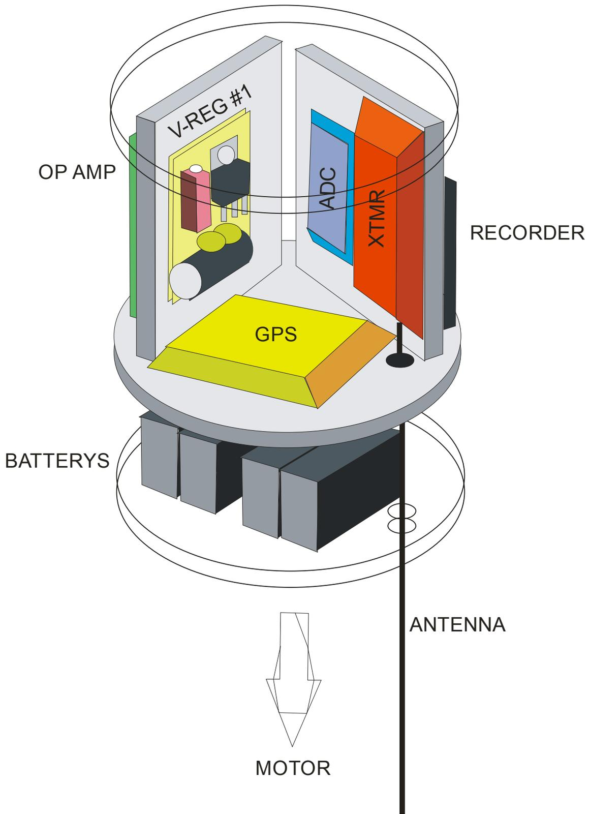
Figure 3.7 Schematic of REMSPEC
