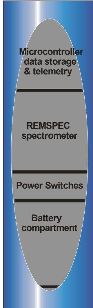
Figure 4.2 Schematic of coupler tube showing arrangement of sub systems.
