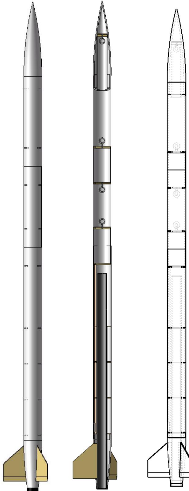
**Figure 3.1: SolidWorks Renderings of the Launch Vehicle**
