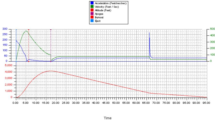
**Figure 3.4: Plots of Simulated Flight Data.**
