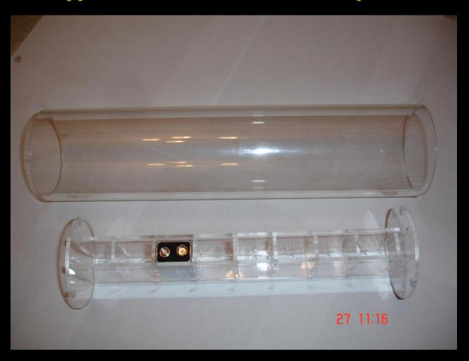
Recovery electronics section: clear acrylic tubing around internal support structure (threaded rods not pictured).
