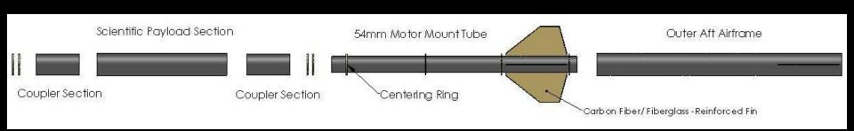
3-D Rendering of Aft Section with SolidWorks 2007
