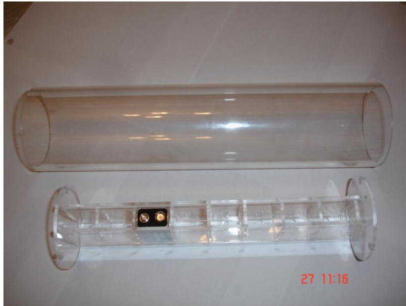
Figure A-7. The outer (3" diameter) clear acrylic tubing with the electronics support board assembly that is housed within in. A 9 volt battery is installed in one of eight battery slots between the two support boards to which the electronics will be attached.
