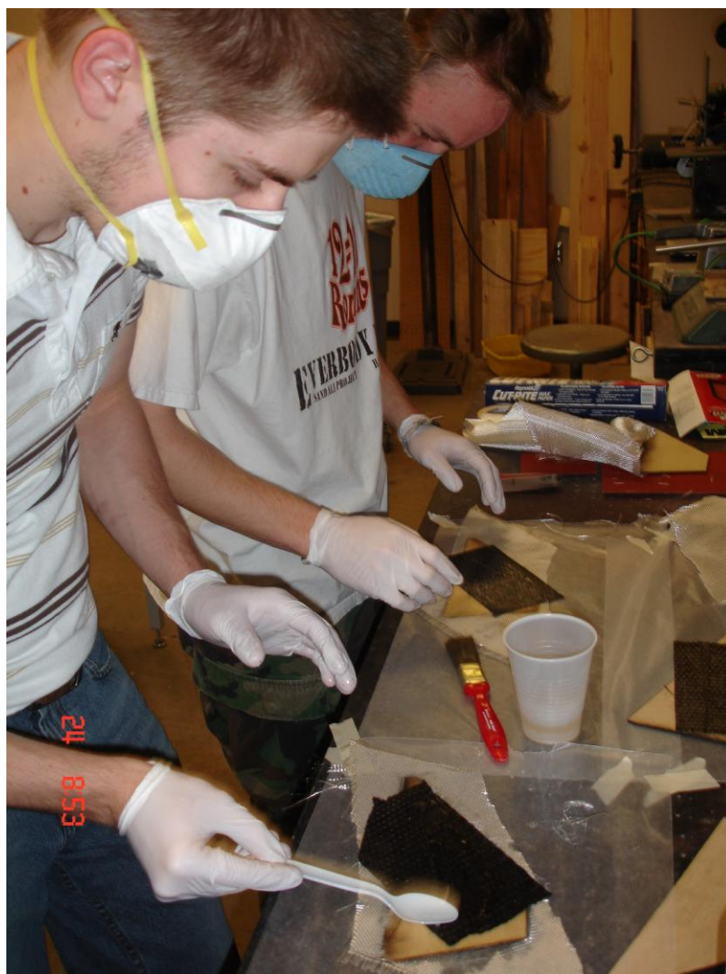
Figure A-2. Aaron Howell (left) and Paul Elliot apply West System epoxy to the fins during the composite fin layup.
