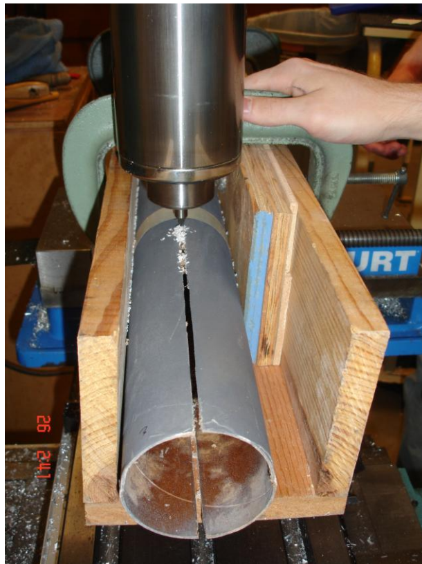
Figure A-6. The slots in the tube are widened and lengthened to accommodate the reinforced fins.
