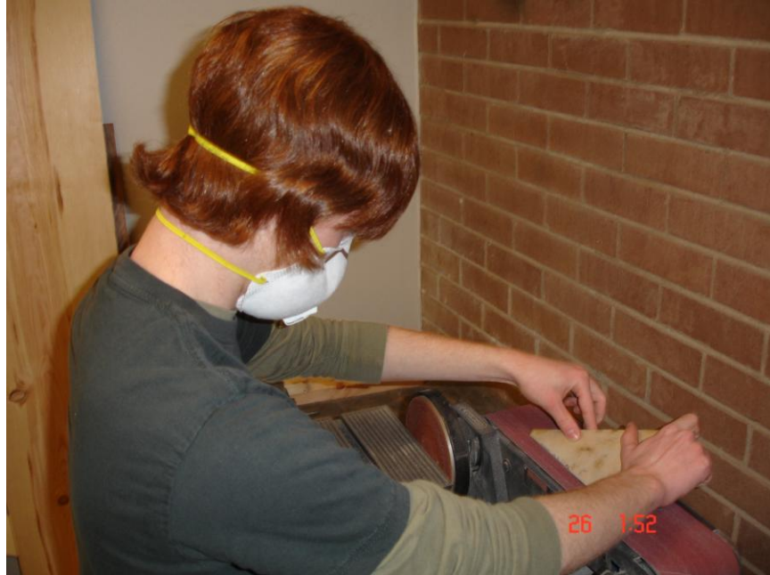
Figure A-3. Greg Lyons uses a belt sander to round the edges of the fins.
