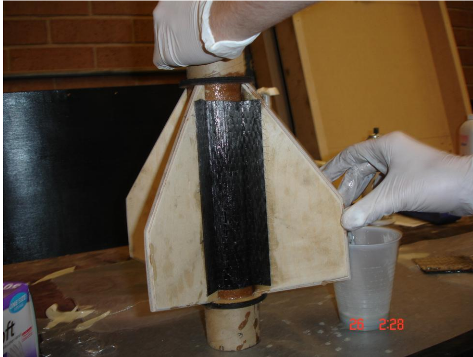
Figure A-5. Carbon fiber was applied from fin to fin across the motor mount tube to make a strong fin can assembly.
