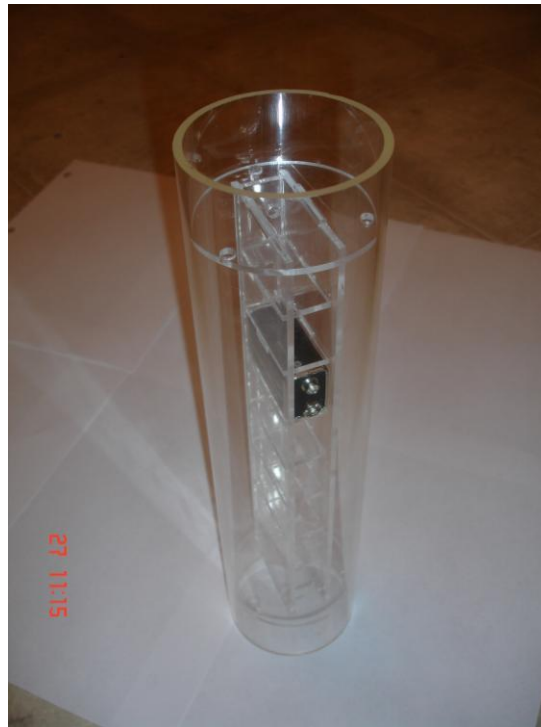
Figure A-8. The clear acrylic electronics support board installed in the 3" diameter clear acrylic tubing. One 9 volt battery is installed in a battery slot between the electronics support board mounting areas.
