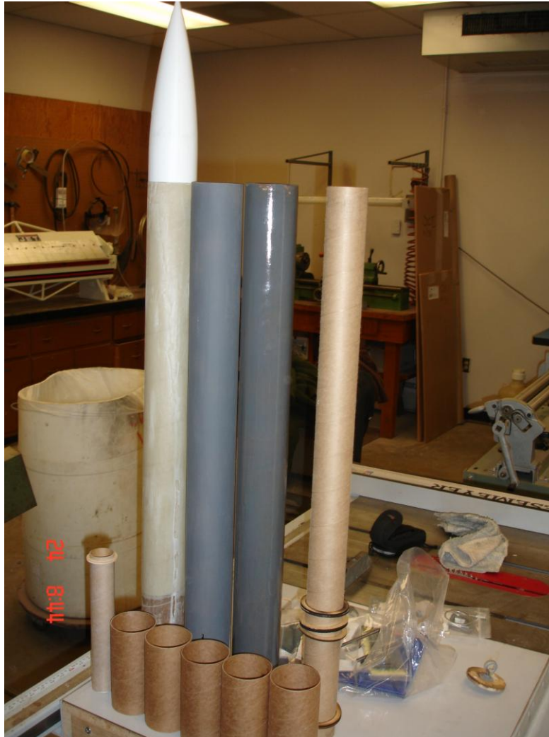
Figure A-1. Major structural components of the competition rocket: (left to right) 38 mm motor adaptor tube, five 3" coupler tubes, the three 34" long 3" diameter main body tubes in varying degrees of finish, and the 34" long 54mm diameter motor mount tube.
